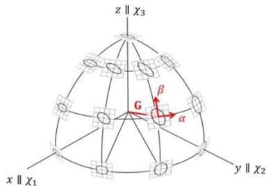
**Fig. 1** Contour maps of  $E(\alpha, \beta) = \text{const.}$  for several reciprocal lattice vectors.
