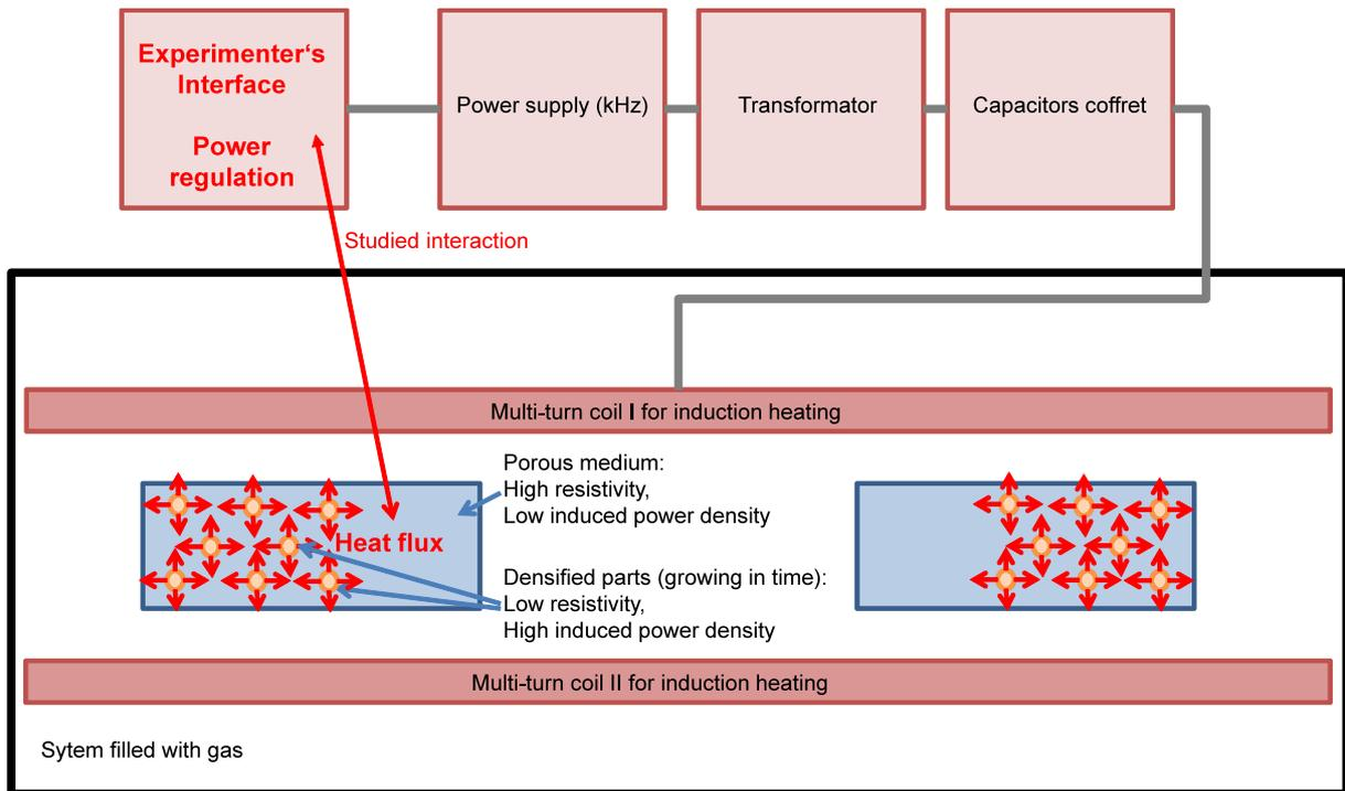
Fig 1: Geometry: Initially porous preform is heated up by induction. The gaseous precursor inside the disc cracks, the disc densifies and changes electromagnetic properties with time. The regulation of the generator has to be adapted to obtain a constant heat flow.
